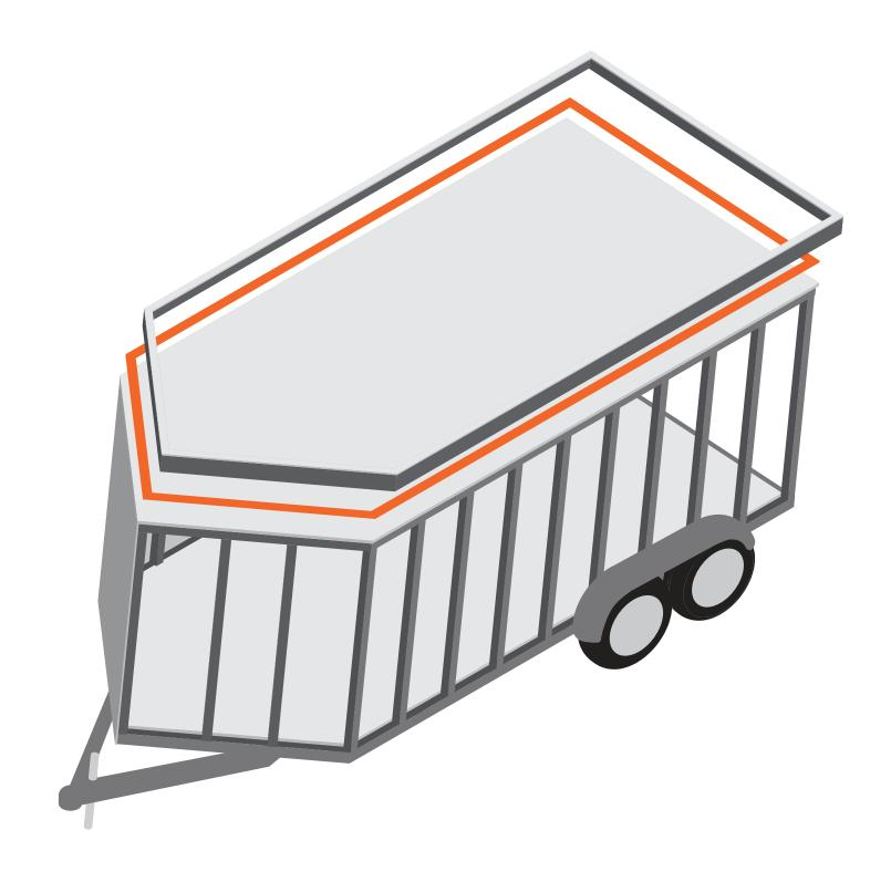
**SEAL BETWEEN ROOF SKIN** AND ROOF WRAP
