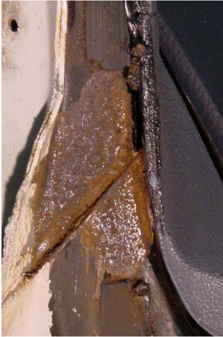
(Level 2 – 3 corrosion of pinchweld)
