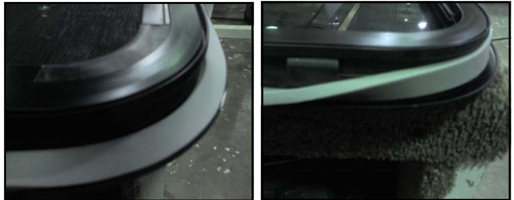
**Seal is rolled on the inside of the flange.**
